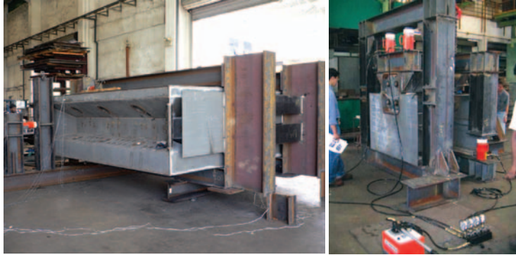
Figure 12. Full-scale prototype load testing
